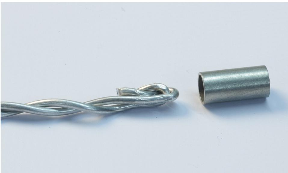
**Doublestrands with 2x1,0mm and 2x1,5mm** should be bend back 180° to create a U shaped loop before being glued into the tubes.
