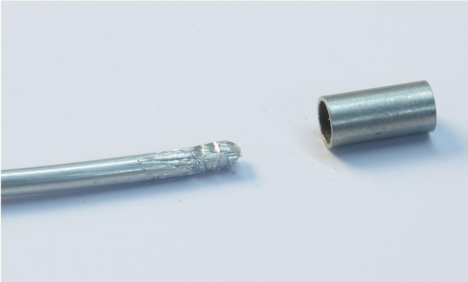
When using thicker **Singlestrands with a diameter from 3.00mm or more** bending the wire back is not possible since the total diameter would exceed the inner diameter of the tube. To prepare these wires squeeze them with some pliers to create some „bite“ marks and to roughen the surface. It is important that these bite marks are only applied to the part of the wire that is later glued inside the tube otherwise
