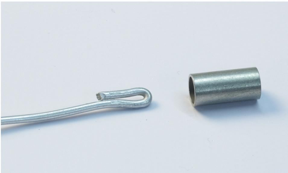
When using a **single strand with a diameter up to 2.5mm** make sure to bend the wire back 180° to create a „U“ shaped loop. Use some pliers to press the loop together in case it won't fit into the tube. Once the glue is set the wire will be secured against turning and getting pulled out of the glue.
