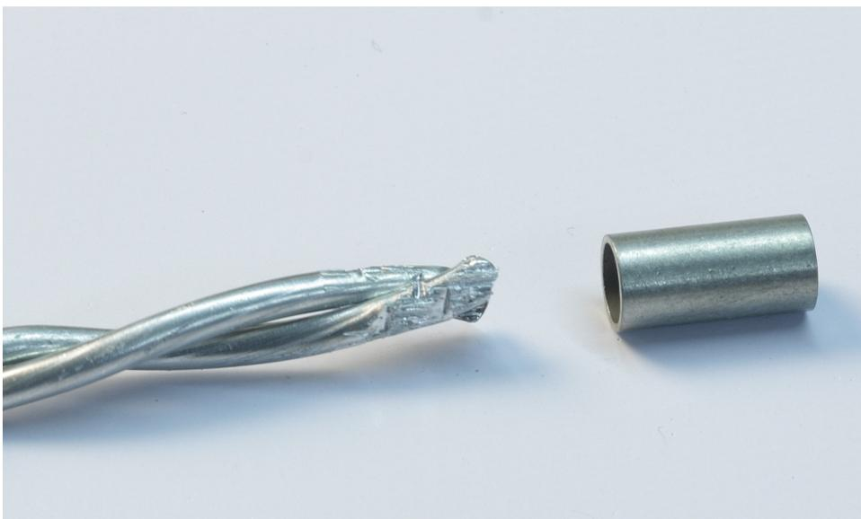
**Doublestrands with 2x2,5mm** can not be bend back at all, the total diameter would exceed the inner diameter of the tube. Clamp these wires with some pliers to create some bite marks and to roughen the surface before glueing them into the tubes.
